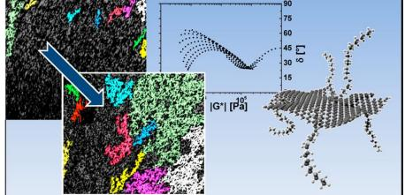
Extensive shear (large amplitude oscillatory shear) led to a destruction of the network while small shear impact (small amplitude oscillatory shear) in combination with elevated temperature was crucial for an effective buildup of the graphene particle network
