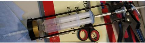
Cartridge press with 2-component syringe and static mixer
